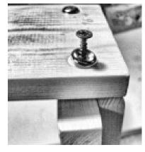
Typical assembly of screw and screw cup. Make sure the screw cup is correct side up.
