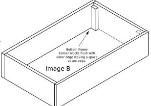
(iii) Repeat step (i) above to fix the remaining top frame long side panel. This will result in a rectangular Bottom Cover Frame. **Image B**.
