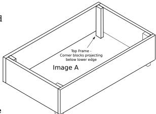
(iii) Repeat step (i) above to fix the remaining top frame long side panel. This will result in a rectangular Top Cover frame. **Image A**.
