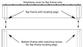
At this stage both Top and Bottom frames will be complete and the top frame locating pegs should engage with the matching recess in the bottom frame. The remaining job will be to fix the top frame polythene cover.
